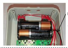
Batteries wires to the right side
