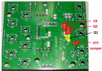
NOTE: The PTT function of Q2 is not installed in this assembly. If that function is required, please see the schematic for wiring connections and create the "PTT Jumper" from one of the legs of Q2, just as it was done with Q1 and solder it in place. Then solder C8, Q2, and trim the leads on Q2.
