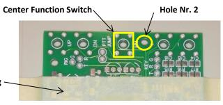
[ ] After the hole is drilled, insert a **4-40 Flat Head** Screw in hole **Nr 2**.
