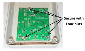
[ ] Remove the four nuts and **PCB** from the Box, but leave the mounting screws in place.
