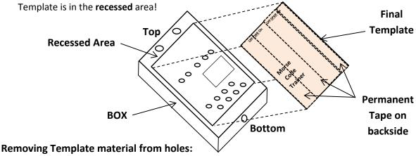
[ ] Using a sharp X-acto Knife, gently push the knife edge down into each hole and follow the edge of each hole to remove the template material from all the round holes in the **Final Template**. Us an **Up and Down motion** to **m**ove the knife around the hole. This will create a clean hole and allow proper clearance for switch access.
