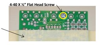
[ ] Apply a **4-40 nut** on each screw inside the box, and Tighten. This will help hold the board in place for the drilling of the remaining holes.
