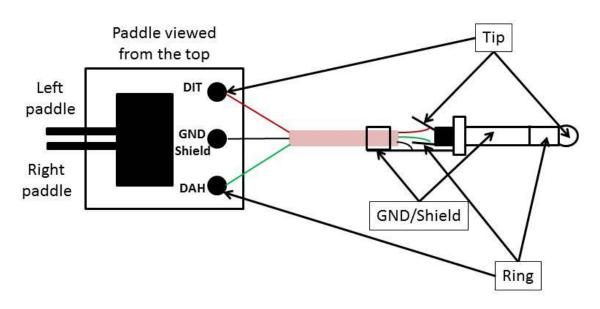
It is recommended that a shielded cable be used to connect the Paddle to the Jack. Use a miniature 1/8 inch Stereo Jack on the end of the cable.
